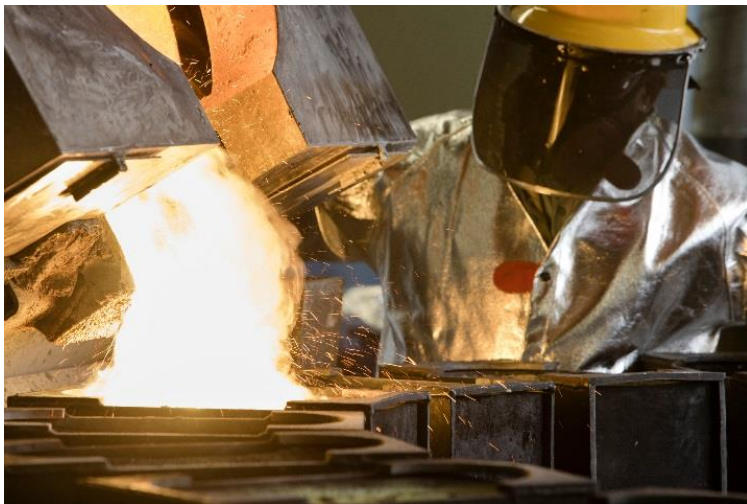
1200 lb Induction Furnace Casting Molten Metal
